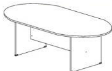
OVAL CONFERENCE TABLE GO 18 1800W x 900D x 750H GO 24 2400W x 1200D x 750H
